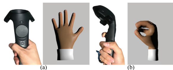
Figure 3: Input processing through combination of controller and virtual hand: (a) default motion, (b) grab motion.
