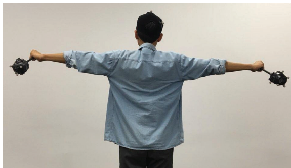
Figure 2. Rowing game equipment. A marker-wrapped hat and a pair of bars recognized as rigid bodies.
