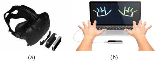
Figure 4: (a) Mounting Leap Motion using VR Mount, (b) Hand motion recognition using Leap Motion
