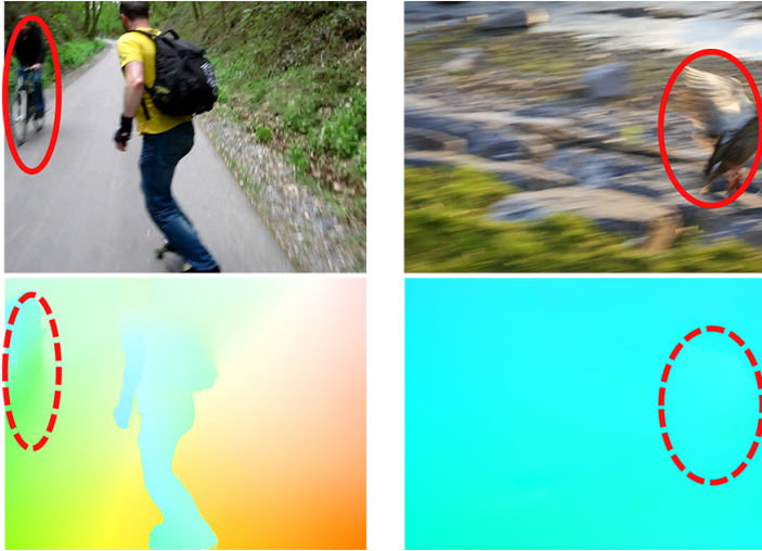
Figure 7: Limitations of our method are demonstrated in failure cases where the whole object exits the frame or the frame experiences severe shaking. In such instances, the optical flow fails to accurately detect these features, highlighting the constraints of our classifier.
