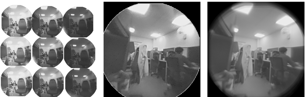
Figure 6: 90 degree FoV Lens: exposure comparison (left), single exposure (middle), and HDR fusion (right).
