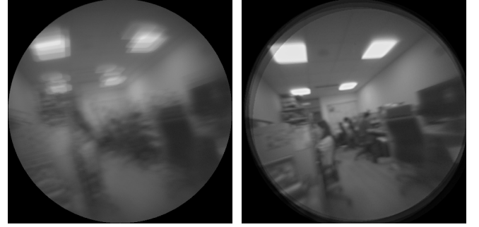
Figure 4: Main lens registration and HDR fusion before (left) and after (right).
