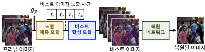
Figure 1. Overview of our pipeline. During inference, the burst synthesis module is removed, and the restoration network processes real burst images captured by real camera system.
