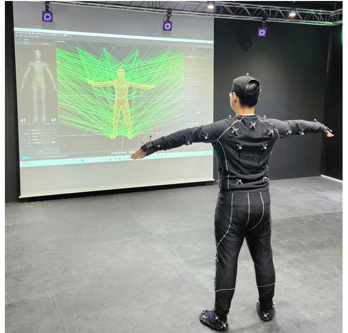
Figure 1. An actor wearing a suit with markers attached and a skeleton is created for human motion estimation in Motive software.
