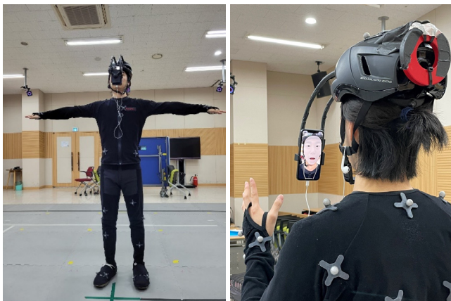
(a) Skeleton calibration (b) Self-made facial capture equipment
